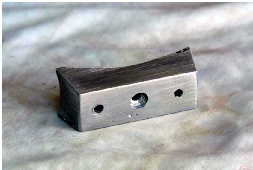
Top View Of Cast Aluminium Mount Block.
