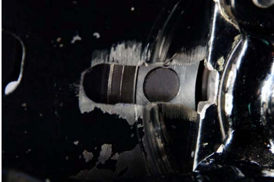
View Showing Backing Plate Sensor Slot In Relation To Magnet.
