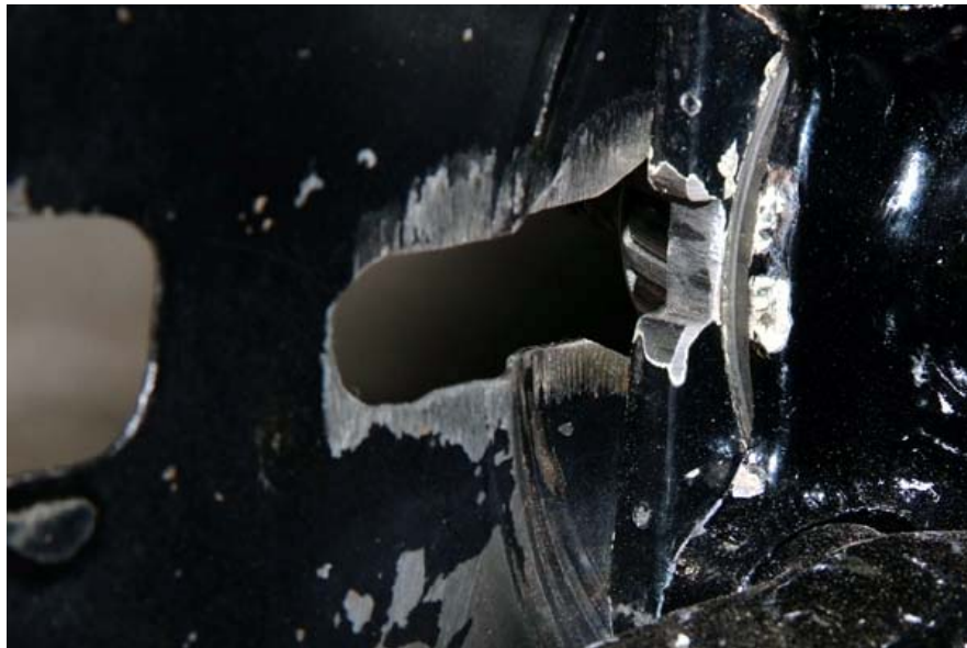
Backing Plate Sensor Access Slot.
