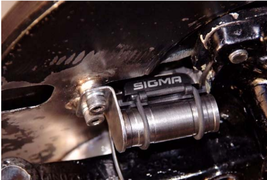
The Sensor Mounted To The Holding Bracket.
