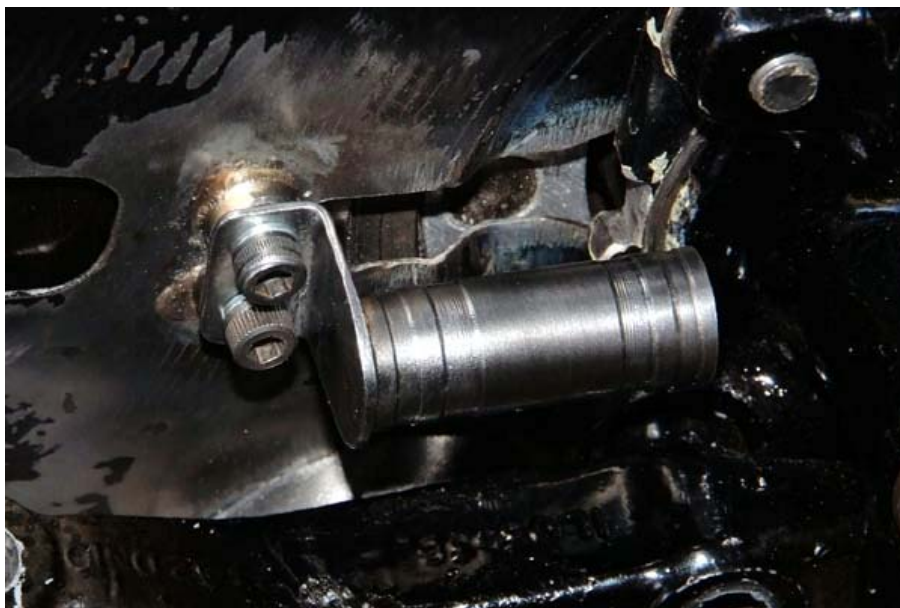
Fabricated Computer Sensor Holding Bracket.
