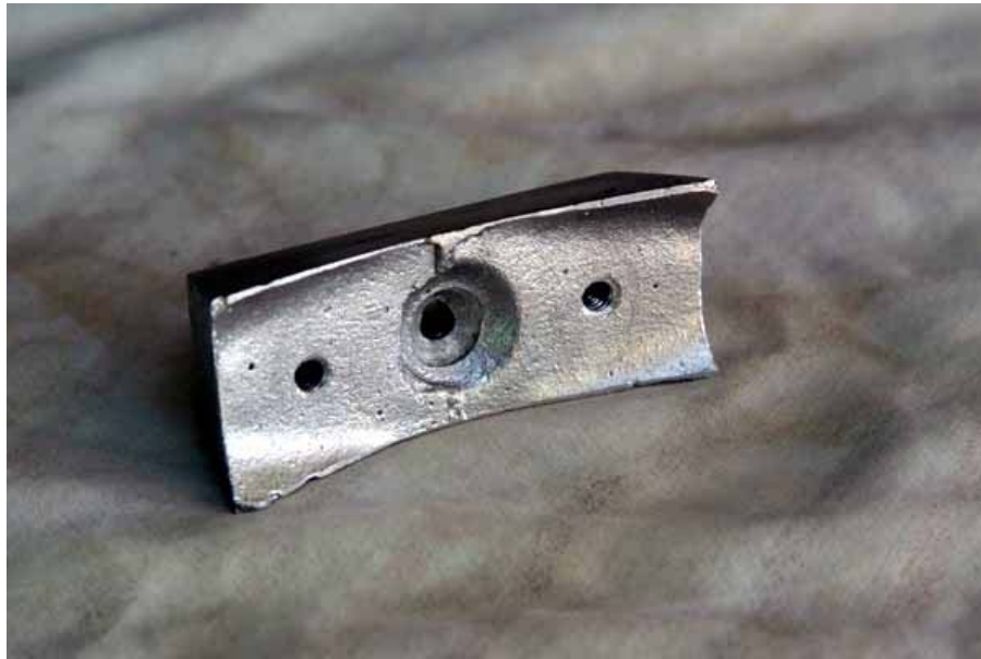
Underneath View of Cast Aluminium Mounting Block.
